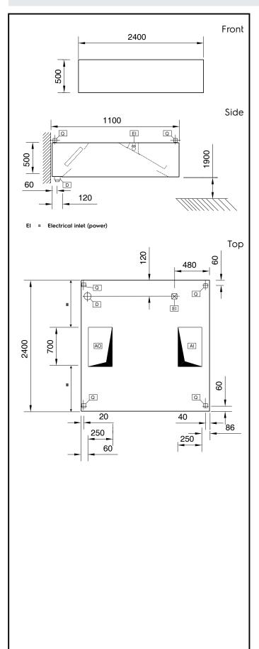
**Electric** Supply voltage: 641252 (STPF1124) 220 V/1N ph/50 Hz **Total Watts:** 0.16 kW Capacity: Supply capacity: 2220 m<sup>3</sup>/h **Key Information:** External dimensions, Width: 2400 mm External dimensions, Depth: 1100 mm External dimensions, Height: 500 mm Net weight: 154 kg Air Emission:
